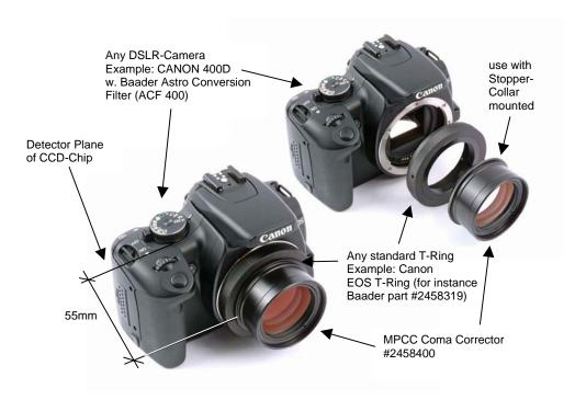
Use without Expansion Ring T-2/M48 to provide 48mm optical length
